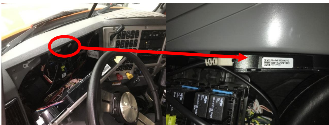
Figure 4. Location of Verizon NetworkFleet 5500 Model in UDOT Snow Plow
